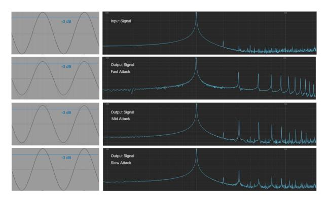
Fast attack adds more harmonics to the output signal compared to the output signal of the slow attack. The distortion occurs due to the non-linear gain applied to the input signal.
