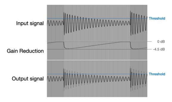
In this example, attack is 1 ms and release is 0.6 s. The initial transient pass through the compressor without gain reduction. It takes a while for the gain reduction to return to 0 dB after the input signal goes below the threshold.
