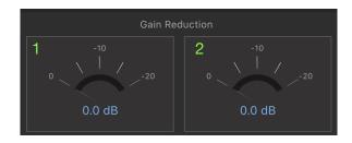
Gain reduction meters shows peak level of the gain reductions in dB.
