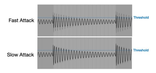
Fast attack makes compressor to start gain reduction immediately after the input signal passes above the threshold. Slow attack, on the other hand, allows many of the transients to pass through compressor without gain reduction.
